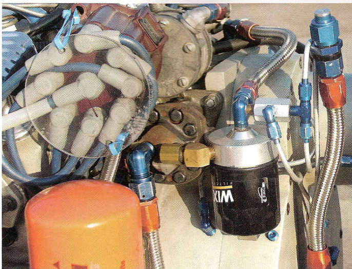
The PSRU lubrication system including oil filter and high-volume oil pump.
