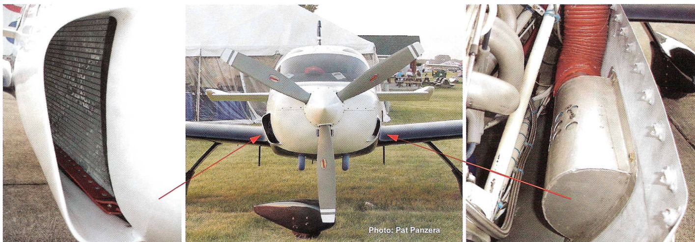
Left: Radiator intake. Middle: Front view of cowl showing radiator inlet and fresh-air scoop. Right: Fresh-air intake.
