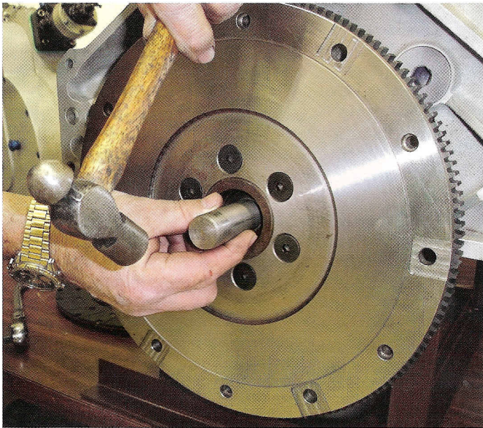
1. After torquing the flywheel in place the pilot shaft bushing is tapped into place.
