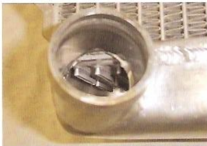
The inside of both tanks are comprised of a series of diagonal, rectangular tubes that allow the flow of coolant from one side of the radiator to another.
